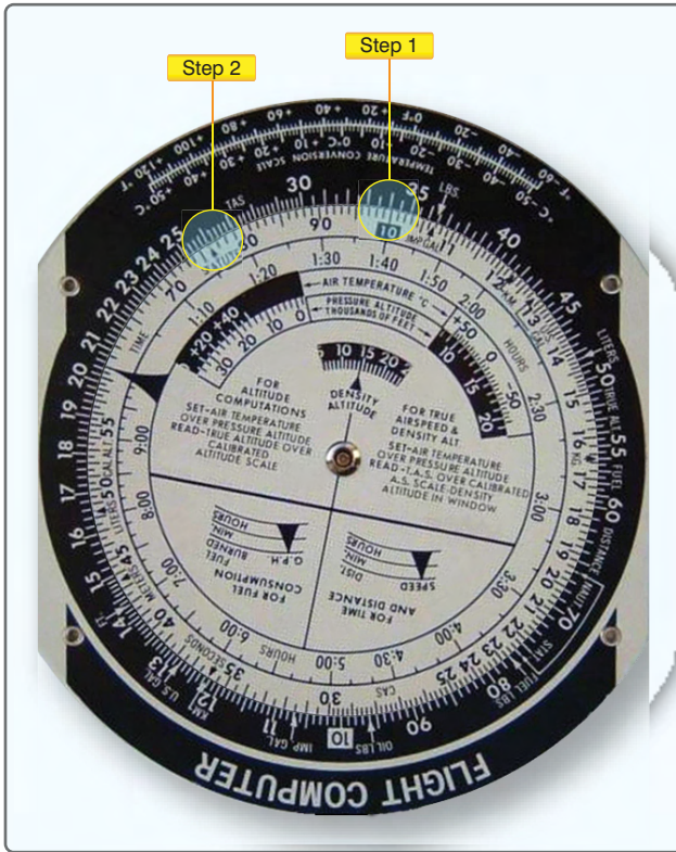
Figure 10-3. E6-B computer set up to multiply 340 by 78.
