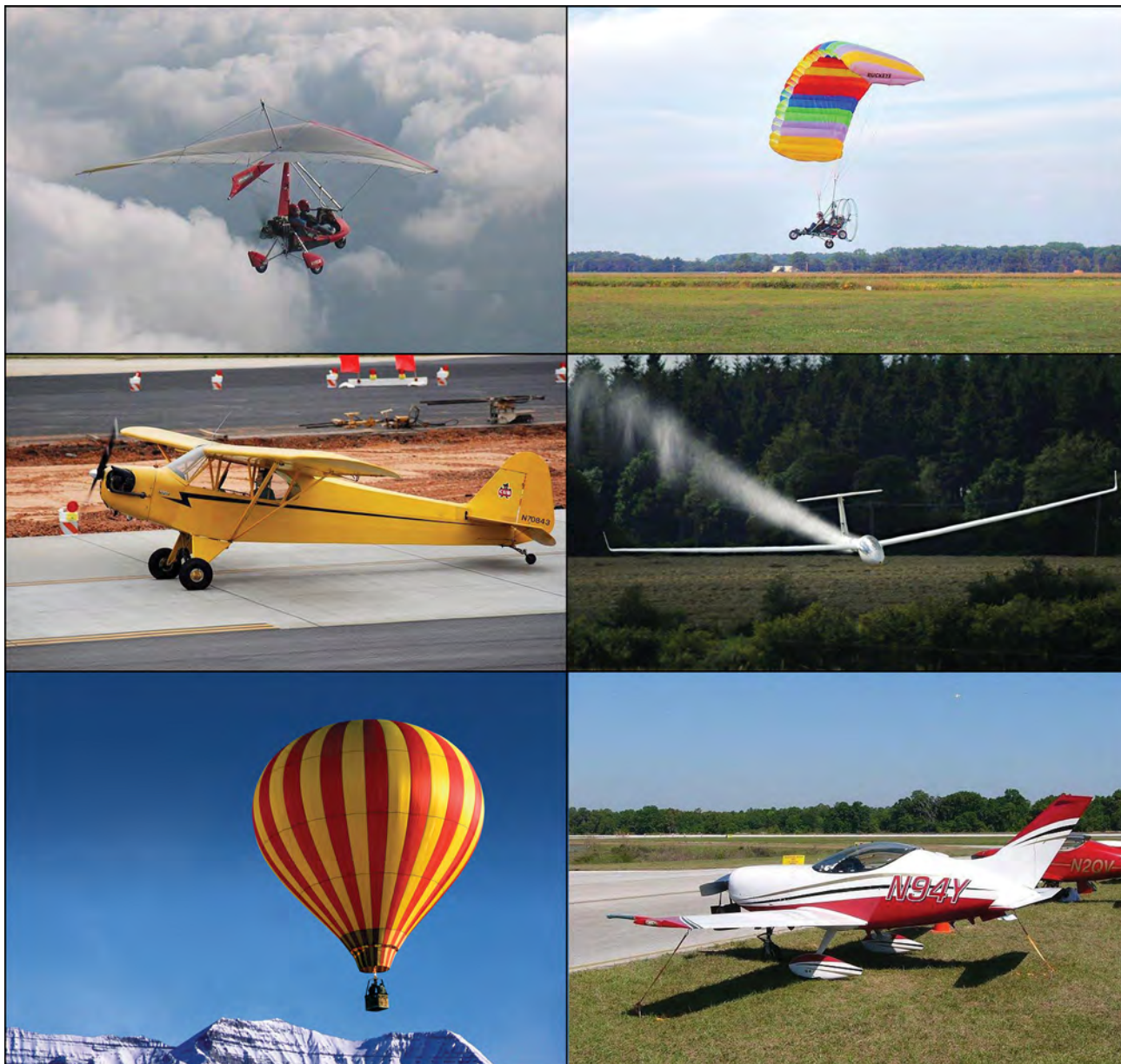
Figure 4-1. Examples of light sport aircraft (from top left, clockwise): weight-shift control, powered parachute, glider, airplanes, hot air balloon, and amateur-built LSA.
