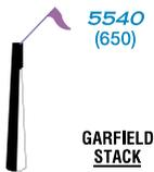
Manmade features used by FAA Air Traffic Control as checkpoints use a graphic symbol shown in black with the required elevation data in blue. The elevation of the top of the obstacle above Mean Sea Level (MSL) and the height of the structure (AGL) is also indicated (when known or can be reliably determined by a Specialist). The AGL height is in parentheses below the MSL elevation. In extremely congested areas, the FAA typically omits the AGL values to avoid confusion.
