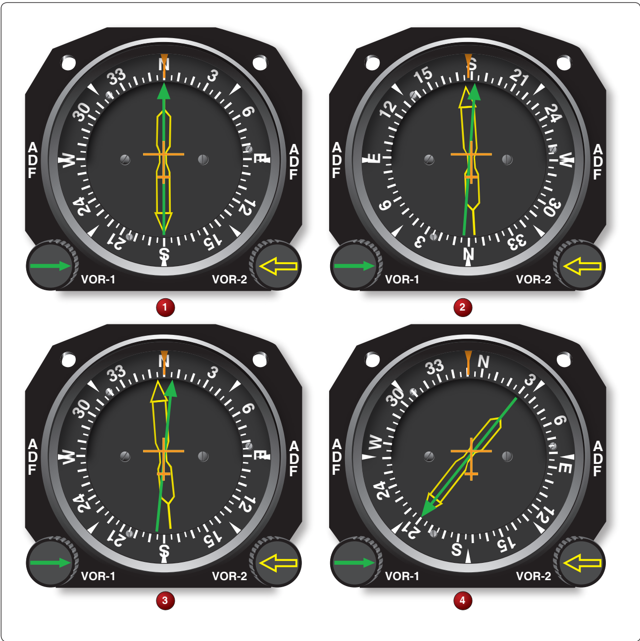
FIGURE 82.—Dual VOR System, Accuracy Check.
