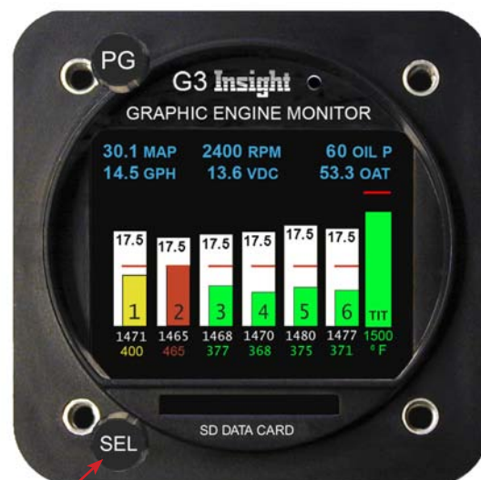
To reset lean function push bottom knob
