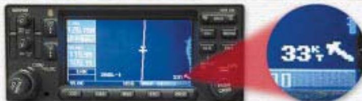
Wind direction arrow with wind speed on the moving map page of Garmin GPS units.
