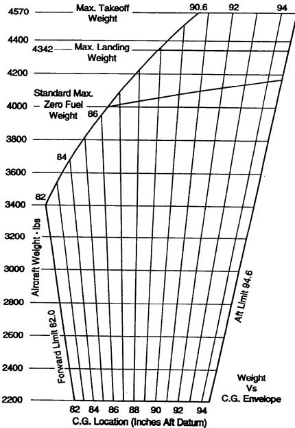
Moment change due to retracting Landing Gear = -32 in.-lbs. C.G. RANGE AND WEIGHT
